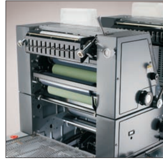
Segmented Lever Actuated Ink Fountains add a great deal of automation for increased productivity and fewer wasted sheets.
