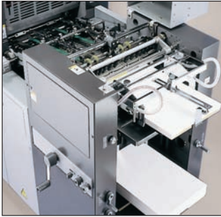
Pre-piling enhances productivity by allowing the operator to preload paper on the lower table while the machine continues to run.
