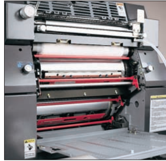
Straight-edge plate clamps with positioning pins are featured. Cylinder safety bars and covers protect fingers.
